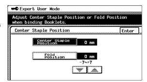
7 If the staple position is too far to the left of the center of the paper, touch to specify the desired positive adjustment (between +1 mm and +7 mm).
